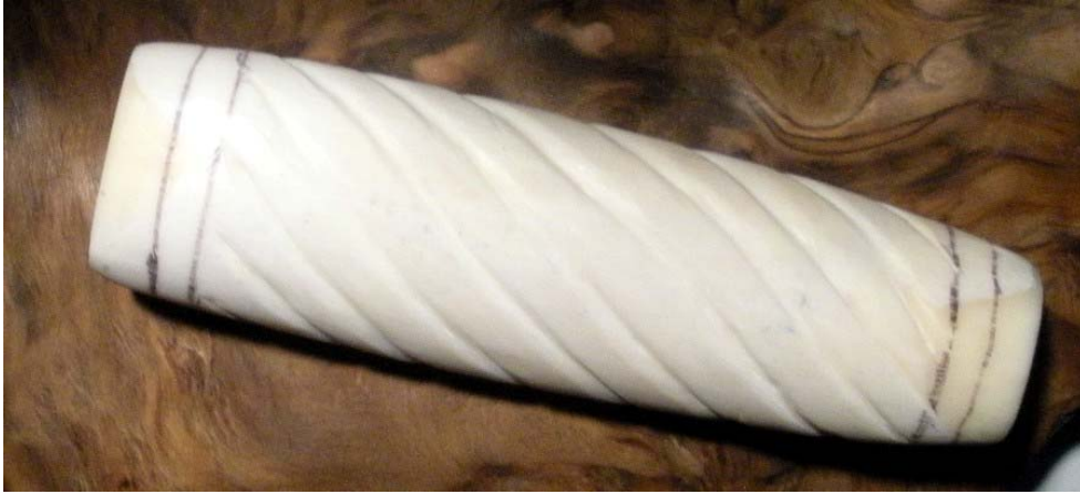
Figure 14 Rough carving of the flutes on the handle
