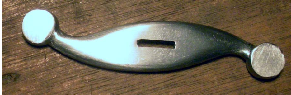
Figure 8 The guard made from scrap 1095
