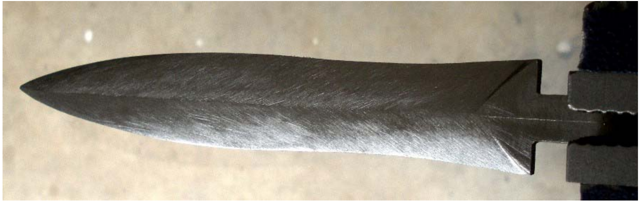
Figure 6 The blade after being roughed out
