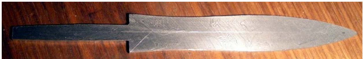
Figure 4 The scribed blade blank
