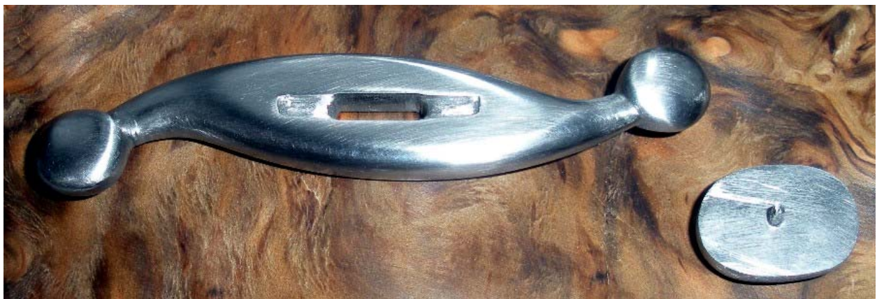
Figure 21 The guard with its blade slot and the pommel with the pin
