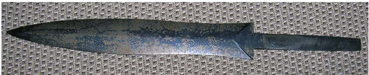
Figure 19 The blade returned from heat treatment
